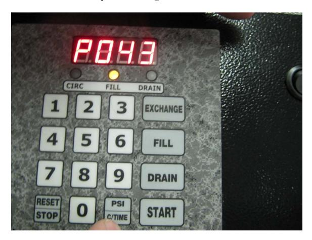
Press PSI/Time Button again this will show Drain Pressure sensor reading. These two reading should be within 2 - 8 lbs of each other
