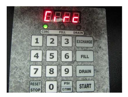
Press Fill 3 0 – Press Start – the pump should be running and then press PSI/ Time button. This will show fill pressure reading.
