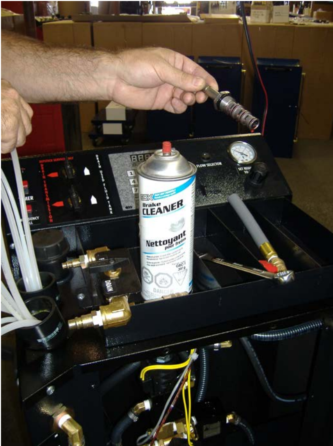
6. Inspect to see if in the plunger a piece of metal is stuck holding it open
