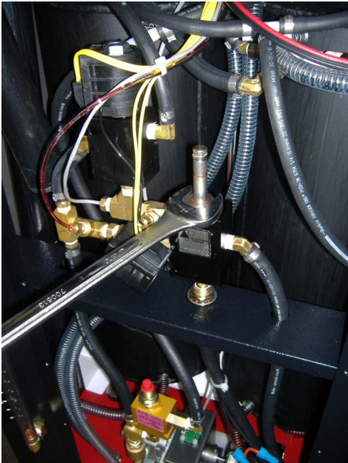
4. With a 1" wrench Remove Cartridge
