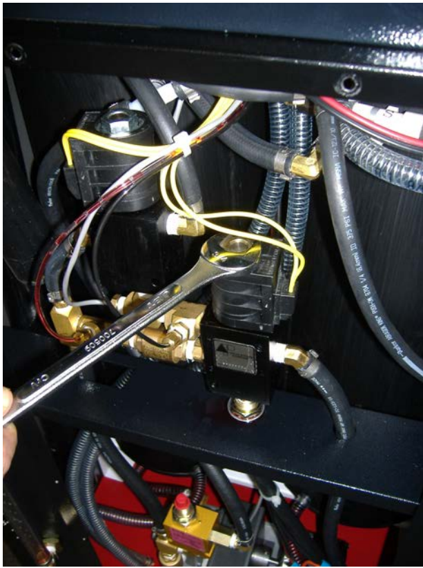
2. Take off nut with a 3/4" wrench. To remove coil pack
